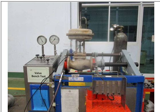
This valve has a seat leakage tested and executed a body pressure test, the result of tested was good.
