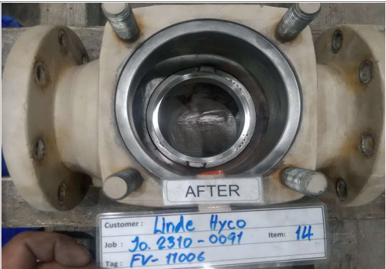
The condition of the inner of valve body after clean and recondition.
